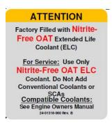
The **new standard coolant** is identified with this sticker. This is the standard coolant of the transportation industry today. It required little or no maintenance and provides superior performance. It, as all coolants, requires regular maintenance to verify freeze protection levels and to verify it has not been contaminated. It does not require that specific SCA levels be maintained. However, this coolant does have some changes that
