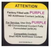
The **previous coolant**, still available as optional, is identified with this sticker. This is a conventional coolant that needed to be maintained every 15k miles with the addition of õSCA¢sö to replenish the depleted additive package provided initially with the antifreeze. This coolant has been in use in the industry for many years and is being replaced as standard with newer
