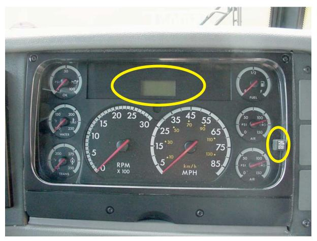
LOCATE THE LCD DISPLAY IN THE CENTER OF THE DASH AND THE RESET'MODE BUTTON TO THE RIGHT.
